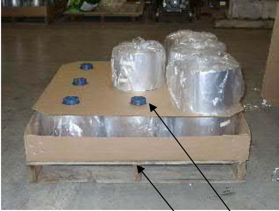
40" x 40" or 48" x 40" Hardwood Pallet Plastic interlocking core plugs (3" core)
